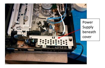
This VCR has a 2pin appliance plug for the mains and the Power-supply is housed in the shielded section closest to the observer. (See photograph above.)
