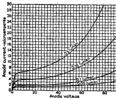
Anode Voltage vs Anode Current
