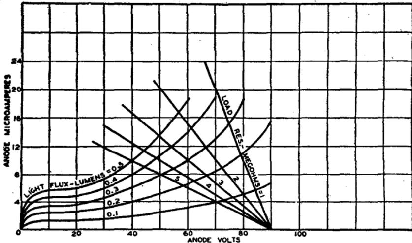
FIG. 7.—Average gaseous type anode characteristics.
