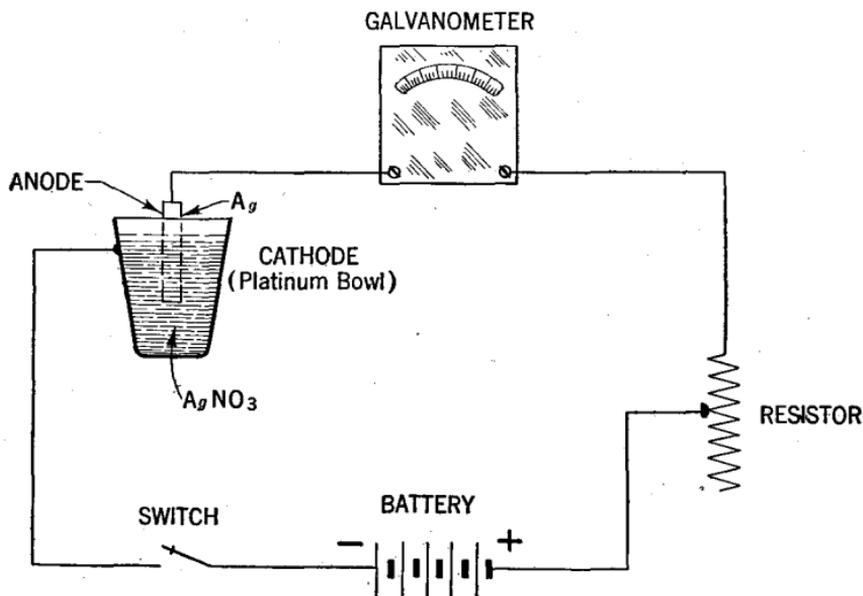
FIG. 5—Diagram of connection to obtain current strength by use of a silver-voltmeter. *Example:* What is the current strength in amperes when after 20 minutes the silver deposit on the cathode is found to be 1.34 gram.
