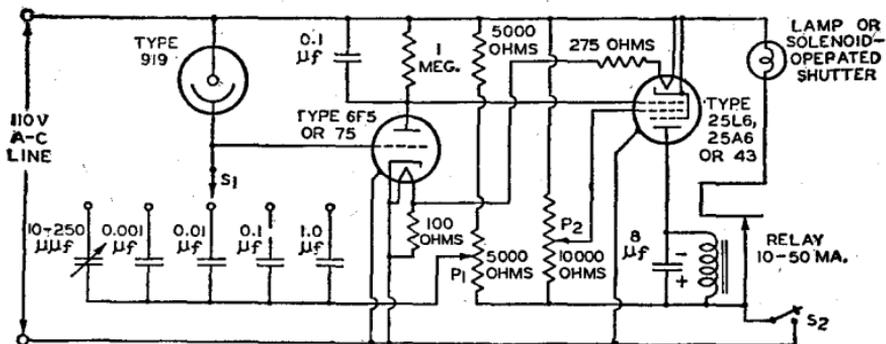
FIG. 20.—A light-quantity metering and control circuit.
