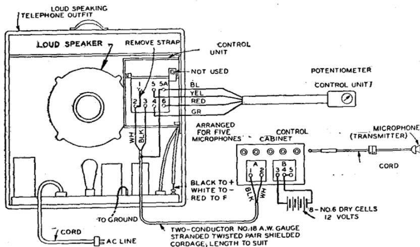
FIG. 2—A small portable announcing system.
