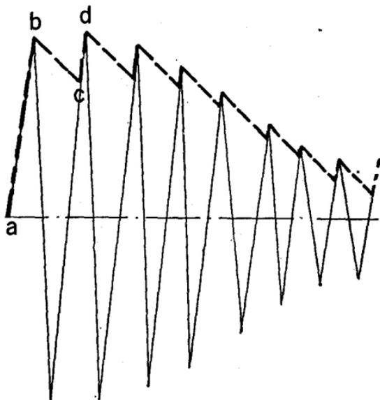
FIG. 22—Diode detector characteristics.
