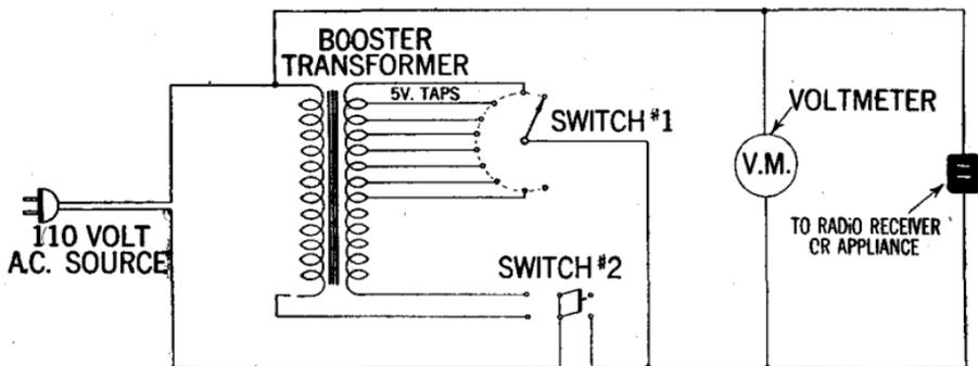
FIG. 17—Schematic diagram of voltage compensating equipment.
