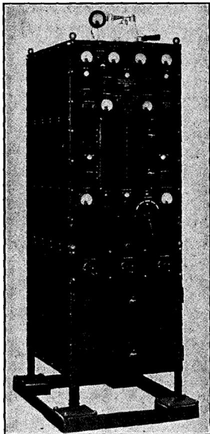
**FIG. 4**—This transmitter operates in the marine wavelength bands between 375 and 500 kilocycles (600-800 meters) and 5,500 to 17,000 kilocycles (17-54 meters). The band from 375 to 500 kilocycles is the one generally
