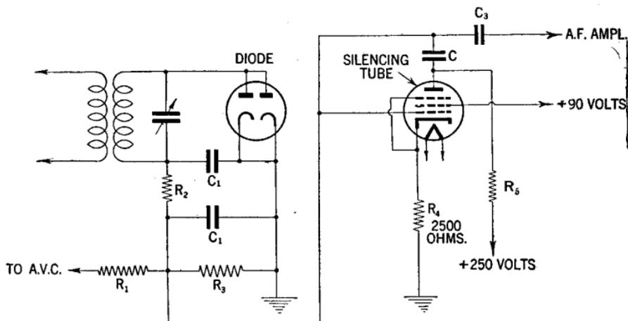
FIG. 14—Automatic tone control circuit.
