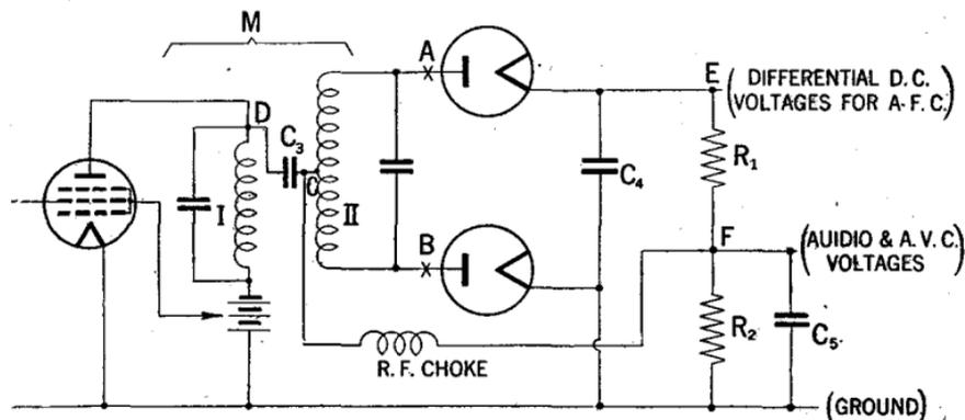
FIG. 3—Automatic radio frequency control detector diagram.
