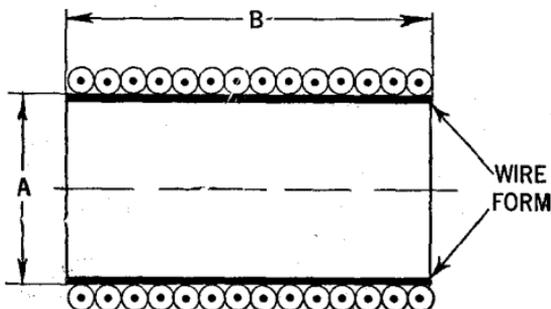
FIG. 1—Cross-section of single layer coil.
