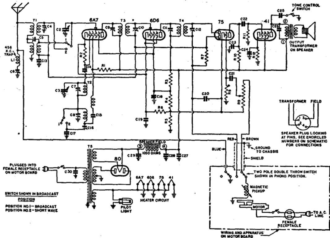
FIG. 20.—Circuit diagram of a 5-tube combination phonograph and dual-wave superheterodyne receiver. (Emerson Model L-143.) *I.f.* peaked at 456 kilocycles. Voltage rating 105 to 125 volts *a.c.* Current drain 0.5 amperes for receiver. Frequency range 540 to 1,750 kilocycles—2,200 to 7,500 kilocycles. Speed of phonograph motor 78 *r.p.m.* at 105 to 125 volts, 60 cycle *a.c.* supply.
