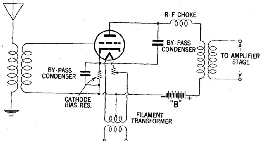
FIG. 25—Grid-biased detector circuit.
