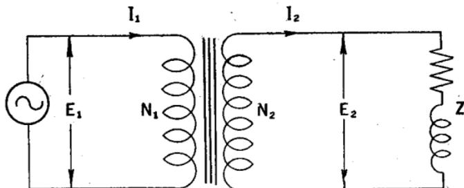
FIG. 4—Simple diagrammatical representation of typical transformer.
