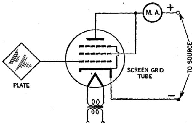
FIG. 36.—Simple circuit for capacity indications.
