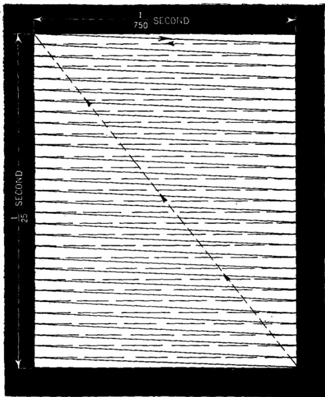
FIG. 17—Simple linear scanning.
