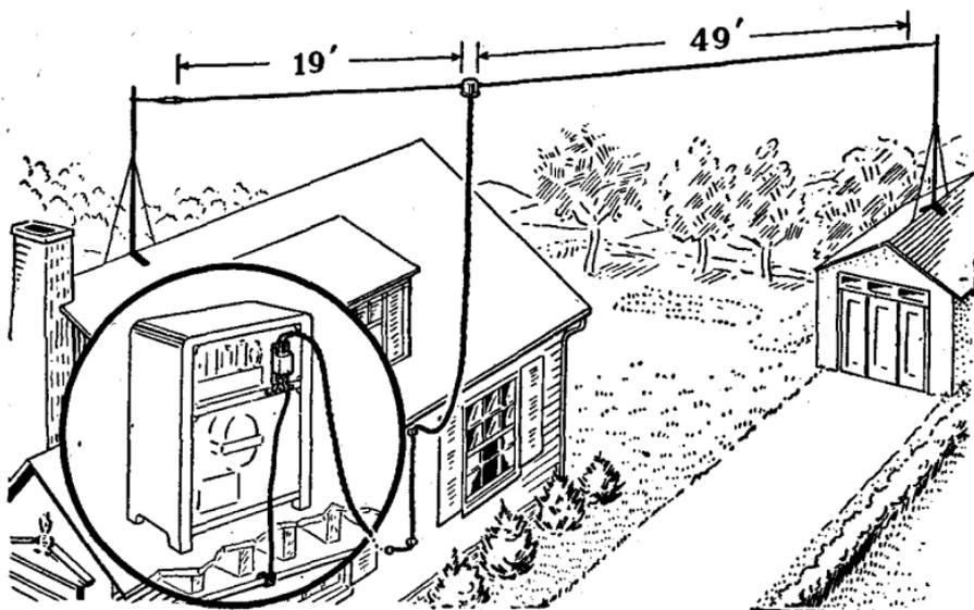
**FIG. 14**—Illustrating how a doublet receiving antenna may be erected. This antenna consists of a special doublet, a transposed transmission line, and antenna junction box and a receiver coupling unit. An antenna of this type is an efficient pick-up medium giving high signal strength over a wide frequency range.
