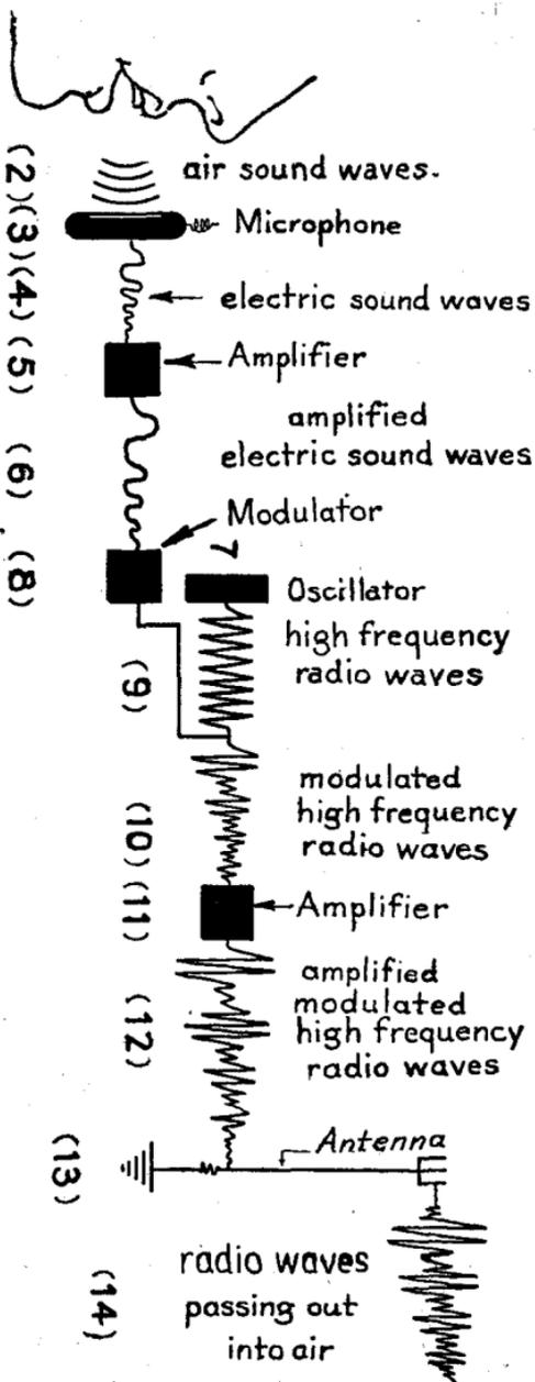
(1) FIG. 3—Schematic illustration of broadcasting principles.
