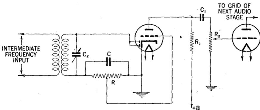
FIG. 23—Diode-biased detector circuit.
