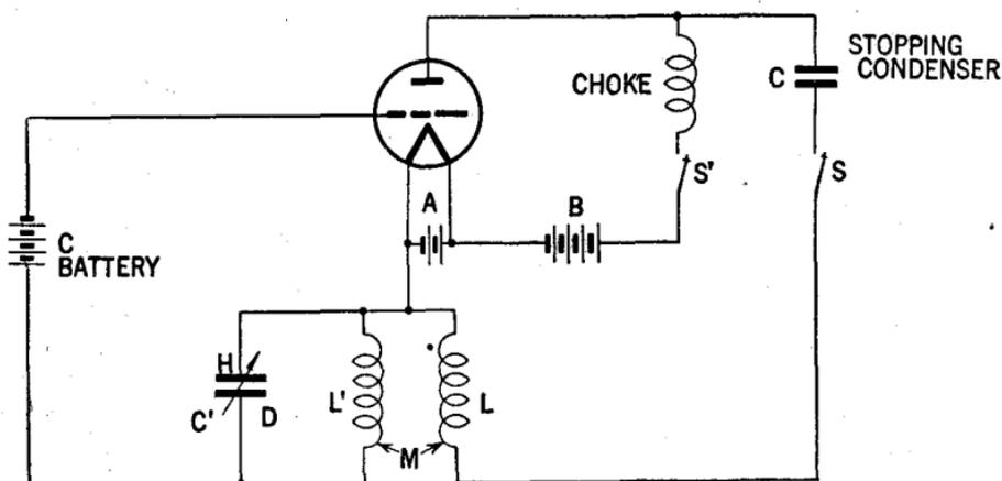
FIG. 6—Modified Hartely type oscillator circuit.
