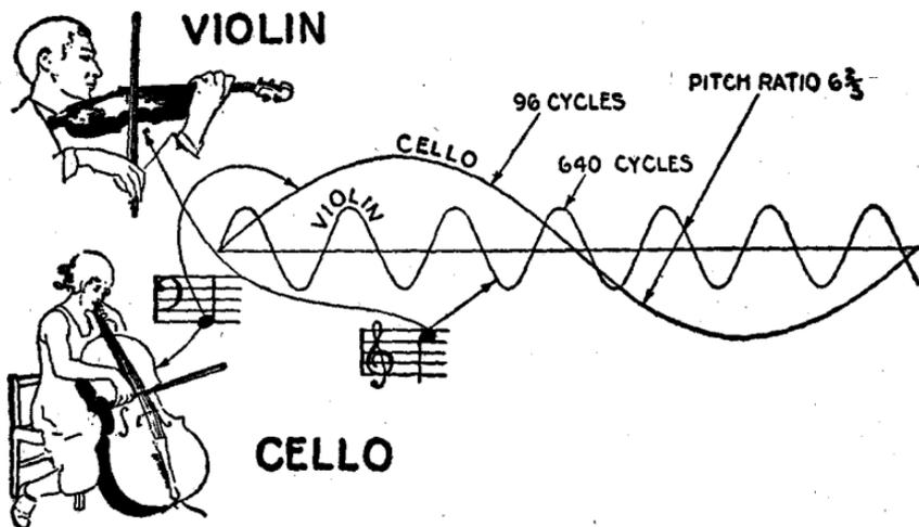
FIG. 9.—Properties of wave motion illustrating *pitch*.
