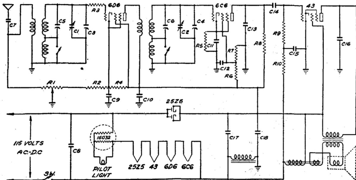
FIG. 17.—Schematic wiring diagram of a 5-tube, 2-band *a.c.-d.c.* radio receiver. (Majestic Model 50.) Operating voltage 105 to 125; *a.c.* or *d.c.* *I.f.* frequency 456 kilocycles. Broadcast band 540 to 1,550 kilocycles. Police band 1,550 to 4,000 kilocycles.
