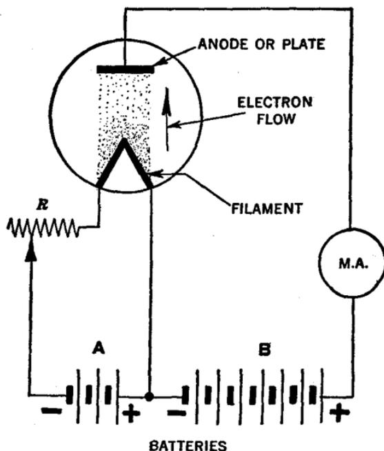
FIG. 10.—Connection diagram for a two electrode tube.
