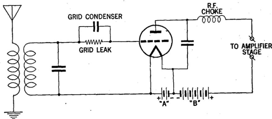
FIG. 26—Detector circuit grid-leak and condenser method.
