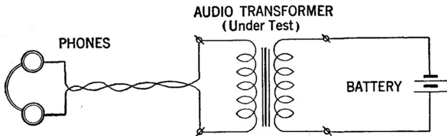
FIG. 18—Method of detecting trouble in audio transformer.
