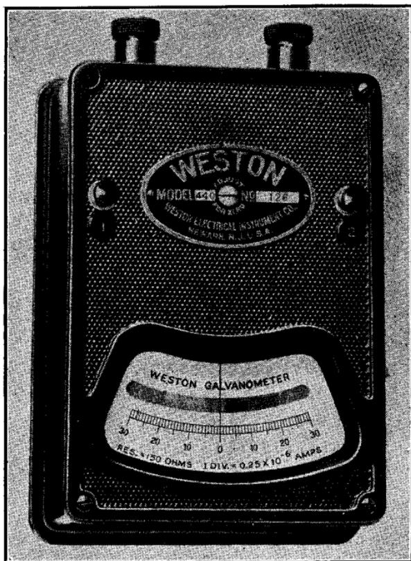
FIG. 4a—Weston model 440 movable coil galvanometer.
