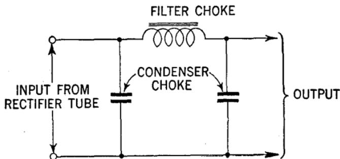
FIG. 7—Condenser-input filter.
