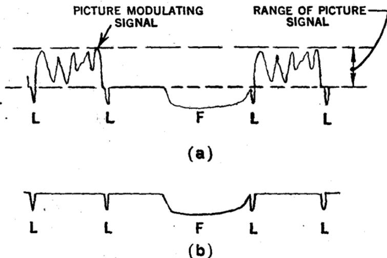
FIG. 19—*a*, composite signal containing picture modulation and synchronizing impulses; *L*, line synchronizing; *F*, picture frame synchronizing; *b*, synchronizing impulses applied to saw-tooth generators.
