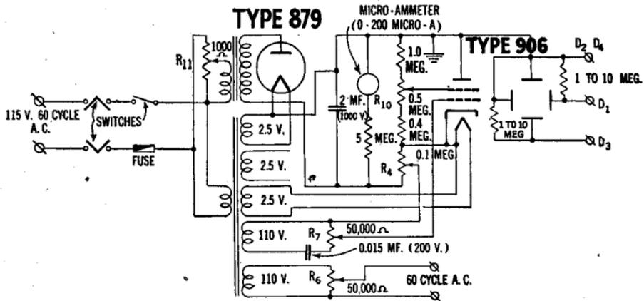
FIG. 10—Typical circuit for cathode ray oscilloscope.
