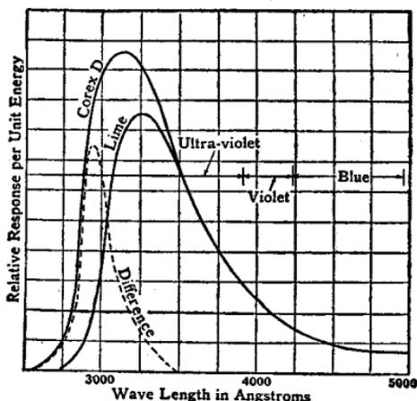
FIG. 12.—Spectral characteristics for a caesium-oxide phototube.
