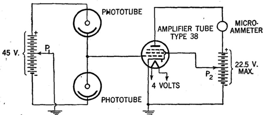
FIG. 22.—Sensitive circuit for matching measurement. Note:  $P_1$  should be set so that with no light on the phototubes, the output-meter reading is approximately mid-scale. Contact  $P_2$  should be set so that the maximum possible output current is limited to 100 microamperes.
