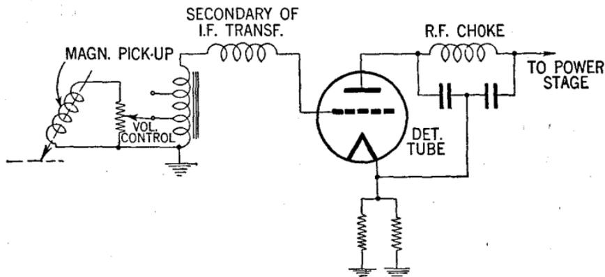
FIG. 10—Method of radio phonograph pick-up connection.
