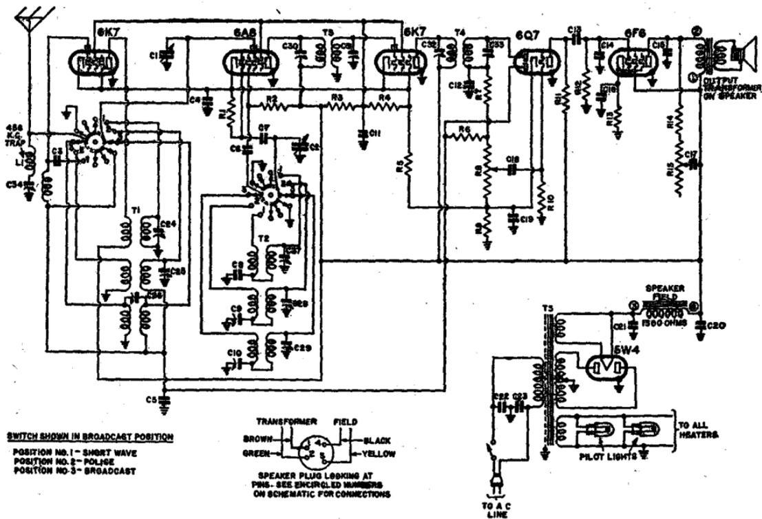
FIG. 14.—Circuit diagram of a 6-tube all-wave a.c. superheterodyne receiver. (Emerson Model S-147, S-151) *i.f.* peaked at 456 kilocycles. Voltage rating 105-125 volts. Current drain 0.55 amperes. Frequency ranges 550 to 1,750 kilocycles; 1,750 to 5,500 kilocycles; 5.7 to 18.0 megacycles.
