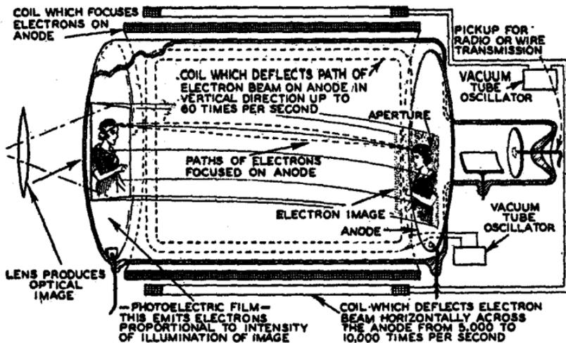
**FIG. 30**—Pictorial diagram explaining the action of the Fansworth television image dissector camera shown on page 592. It should be noted that the number of scanning lines is the horizontal frequency divided by the vertical frequency or  $\text{Lines} = \frac{\text{Horizontal frequency}}{\text{Vertical frequency}}$
