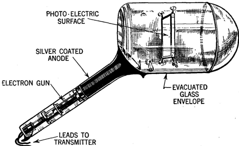
FIG. 11—Another type of cathode ray transmitting tube.
