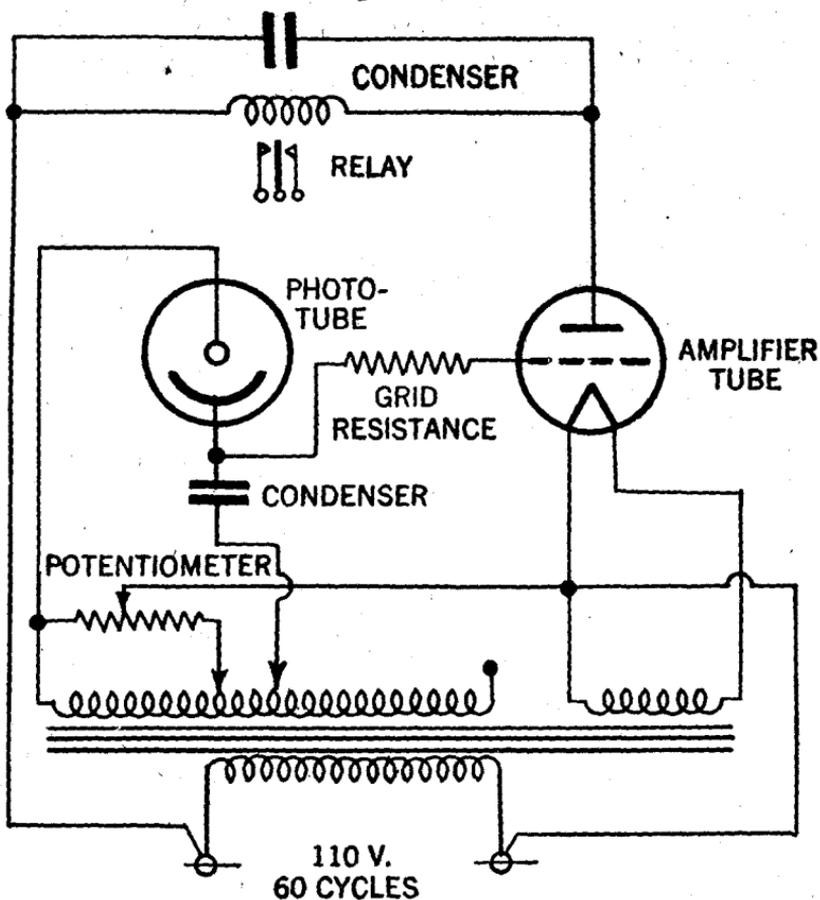
FIG. 48.—Simple amplifier for straight A. C. operation.
