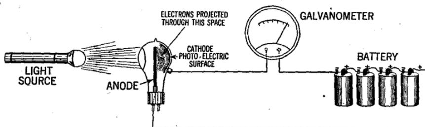
**FIG. 2**—To increase the amount of deflection (efficiency of light conversion) various methods of current amplification similar to that associated with current amplification in radio circuits is employed.
