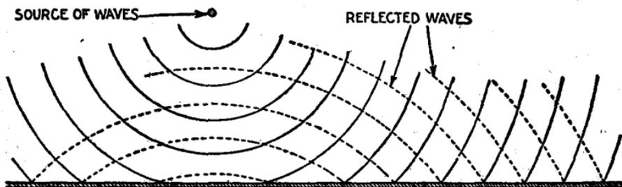
FIG. 5.—Reflection of waves from a plane surface.
