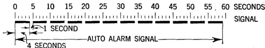
FIG. 1—Standard auto alarm signal.
