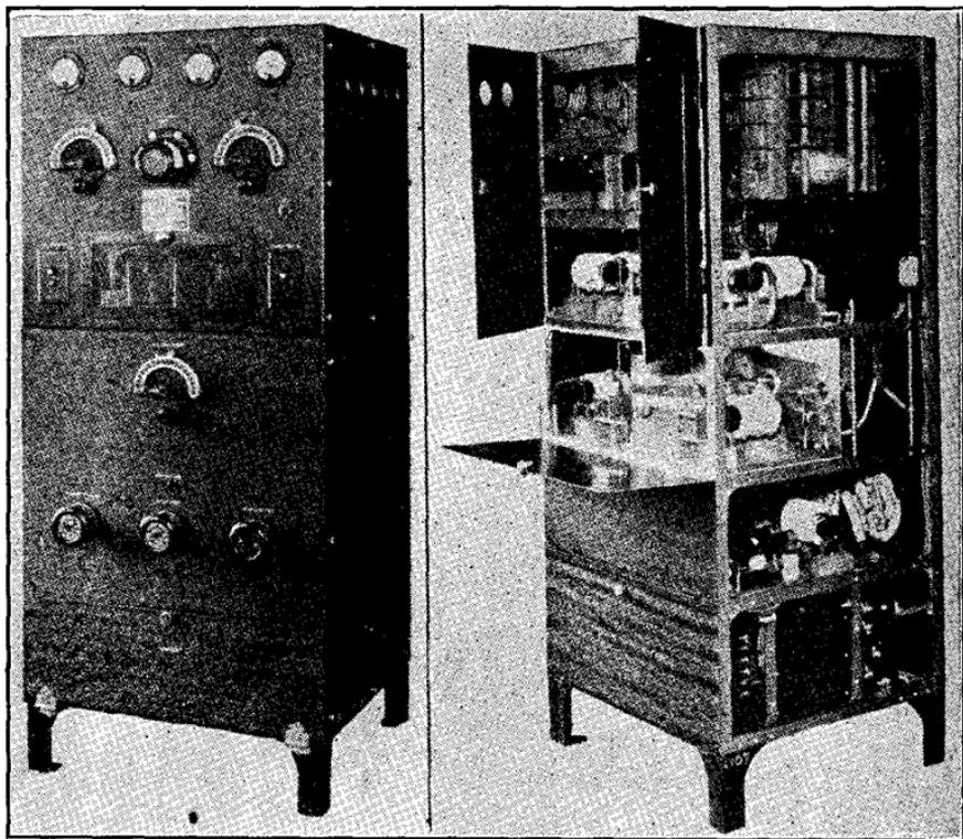
FIG. 2—Standard 200 Watts Marine Radiobeacon transmitter.
