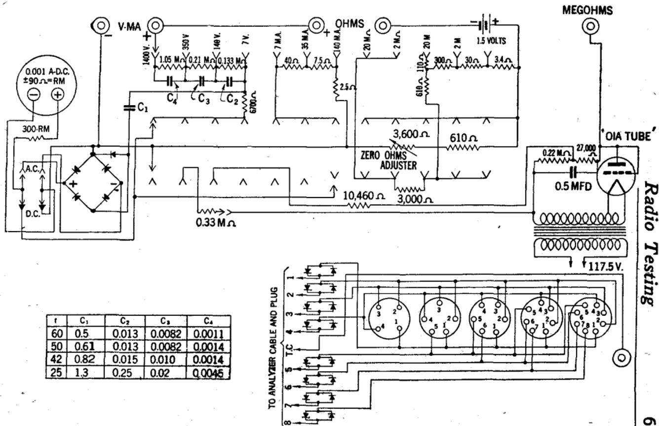
FIG. 27—Wiring diagram of Supreme Model 551 analyzer.
