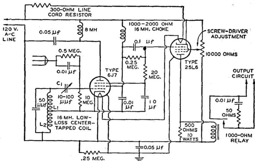
FIG. 38.—Self-balancing capacity-operated relay.
