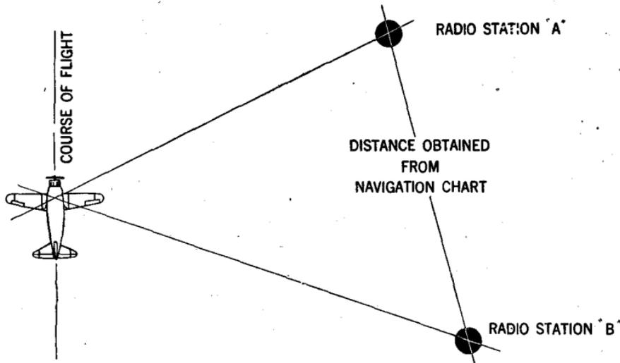
**FIG. 6**—Illustrating method of determining position by means of radio compass. As the surrounding territory shown on air navigation chart is laid out in scale, it follows that the intersection of the two lines gives the approximate location of the aircraft. It is evident that the accuracy of position so obtained will depend on such factors as: flying speed; angle and distance between aircraft and stations; accuracy of instruments; skill of navigator, etc.
