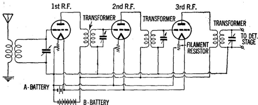
FIG. 14—Three stage radio frequency amplifier circuit.
