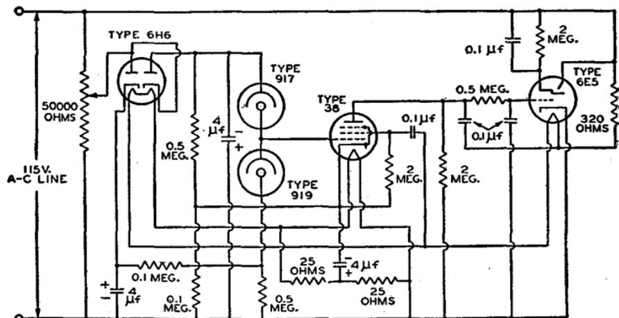
FIG. 21.—A sensitive light-balance indicator.
