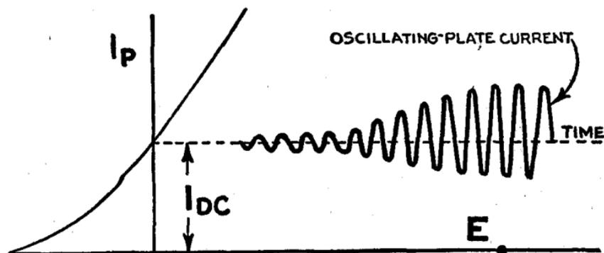
FIG. 7—Oscillating plate current characteristics.
