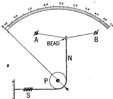
FIG. 16.—Simplified diagram illustrating the construction of a hot wire instrument. *N*, represents a silk thread connected to spring *S*, wound around pulley *P*, and attached to a bead threaded on wire *AB*. Wire *AB*, made of platinum alloy, is connected in the circuit whose current is to be measured. This wire lengthens, due to the heating effect ( $I^2R$ ) when a current flows through it. The slack is taken up by spring *S*, causing pulley to turn and move the pointer over the scale.
