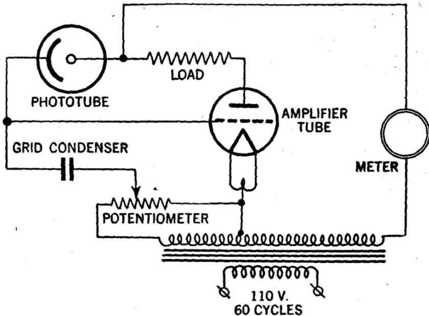
FIG. 46.—Simple amplifier for straight A. C. operation.
