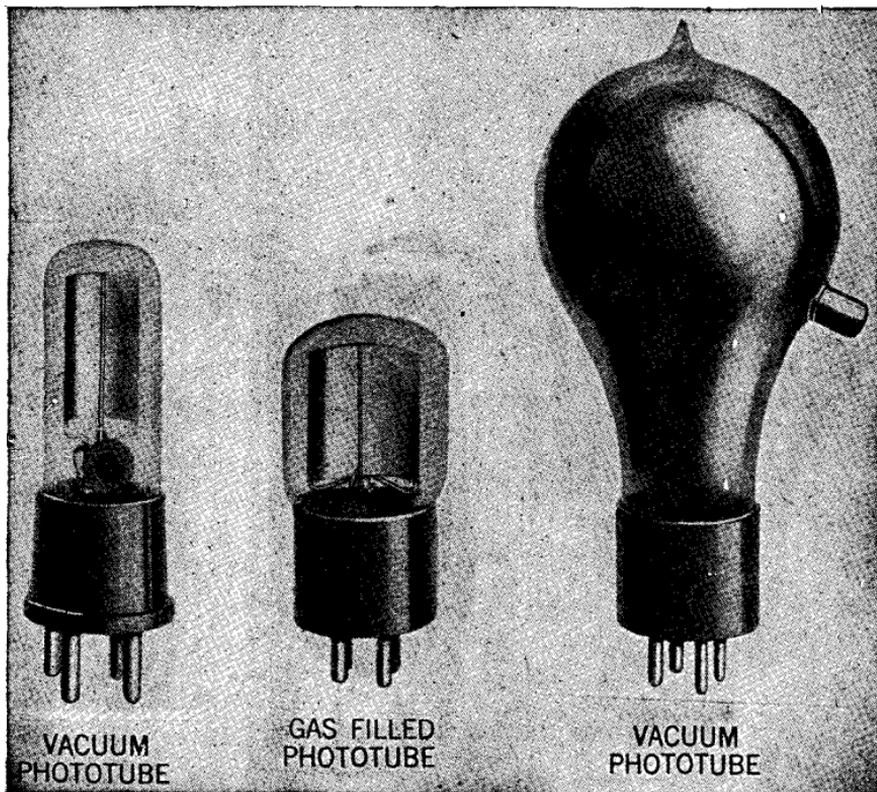
FIG. 5.—Typical phototubes.
