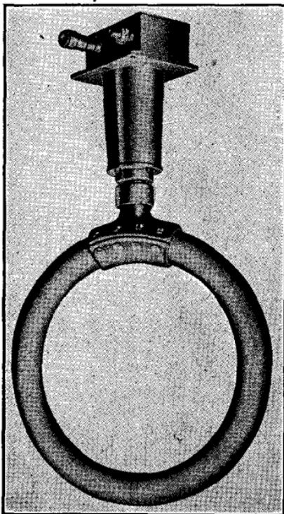
FIG. 8—Aircraft loop-antenna. (Courtesy Western Electric Co. Inc.)
