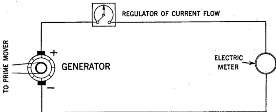
FIG. 7.—Note the similarity to the hydraulic circuit.
