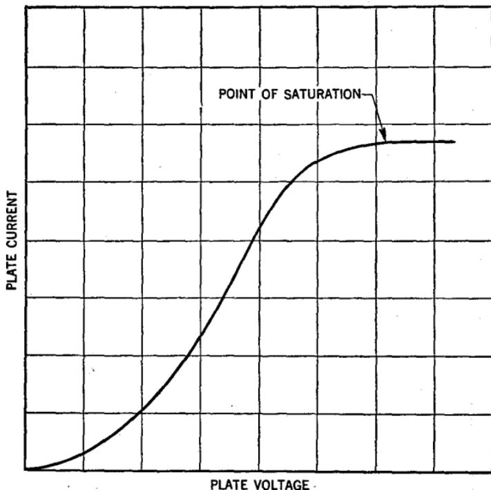
FIG. 13.—Characteristic curve of a diode.
