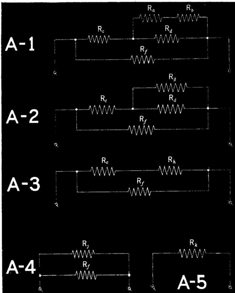
Method illustrating how a series parallel resistance combination of type shown in A-1 may be reduced to the simple form of that shown in fig. A-5.
