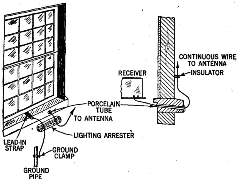
FIG. 8—Conventional method of installing inverted L-antenna lead-ins.
