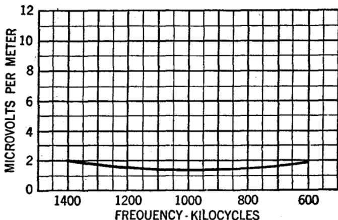
FIG. 7—Typical radio receiver, sensitivity characteristics.
