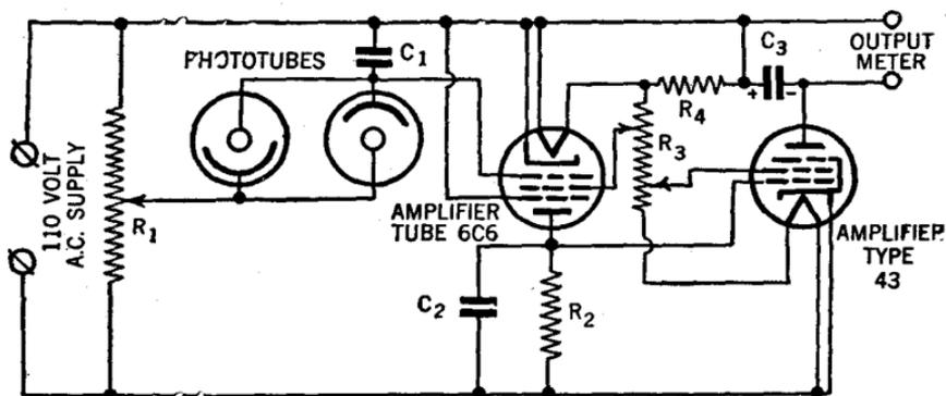
FIG. 25.—Circuit for measurement of light intensity ratios.
