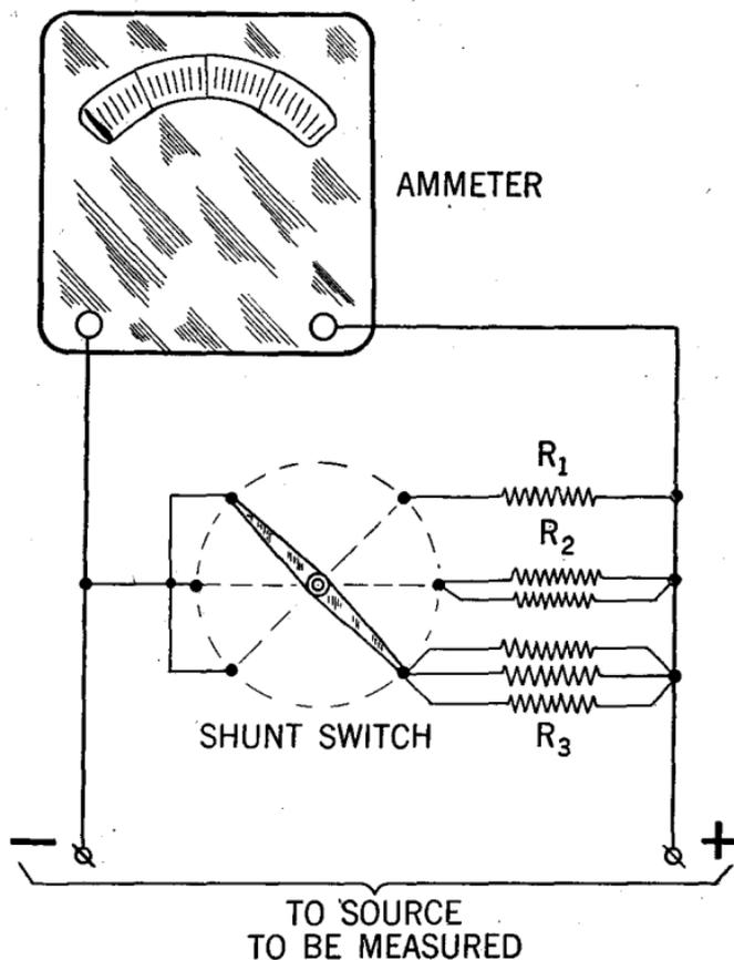
**FIG. 14**—Arrangement in which shunts  $R_1$ ,  $R_2$  and  $R_3$  may be utilized for various size current measurements. In the case where the meter has only one scale, current indication shown on meter should be multiplied by the value of the multiplication factor given for each shunt.
