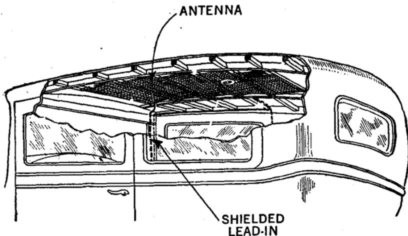
**FIG. 2**—Illustrating location of roof type antenna.
