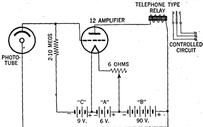
FIG. 42.—Simple battery operated amplifier.
