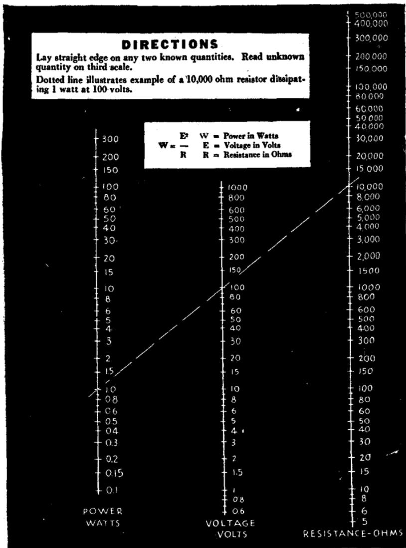
FIG. 24—Convenient table giving the scalar relation between resistance ( $R$ ), voltage ( $E$ ) and power ( $W$ ). With the chart and a straight edge any of the above quantities can be determined if the other two are known.
