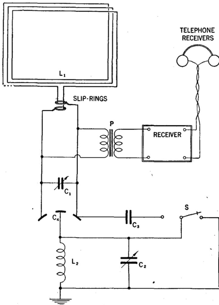
FIG. 4—Circuit of Kolster radio direction finder.
