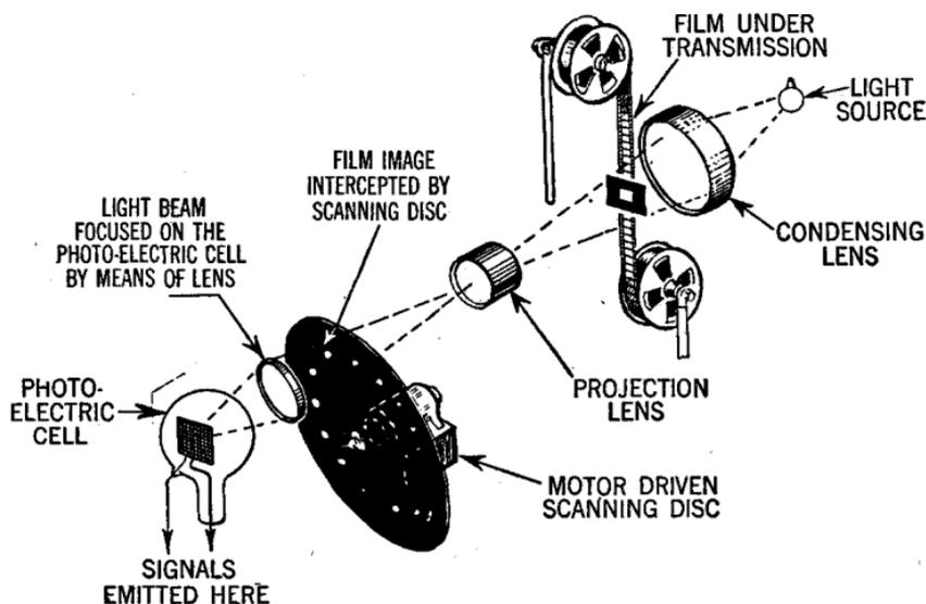
FIG. 4—Simplified view of a mechanical transmitting system.
