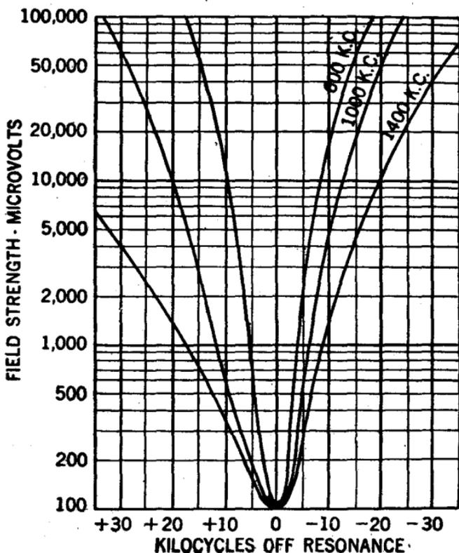
FIG. 5—A typical radio receiver selectivity curve.
