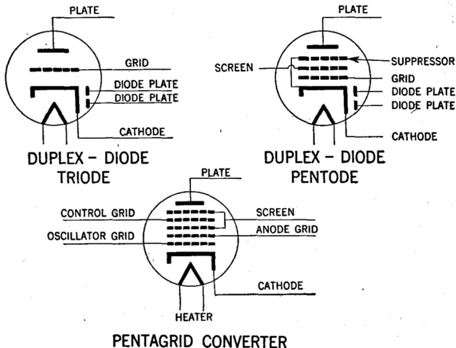
Figs. 21 to 23.—Schematic representation of multi-purpose tubes.
