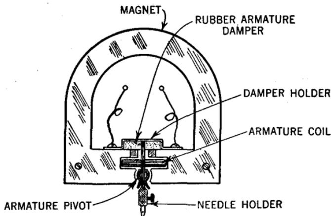
**FIG. 2—**Principal parts of a rubber damped magnetic pick-up.
