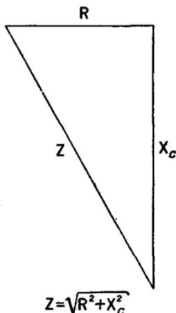
FIG. 21—Arrangement of impedance triangle in capacity measurements.
