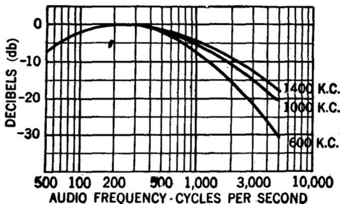
FIG. 8—Typical radio receiver, fidelity characteristics.
