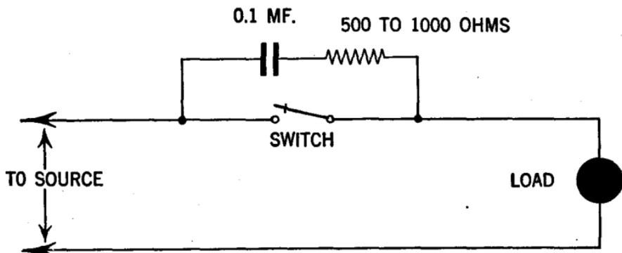
FIG. 6—Method of filter connections across switch.
