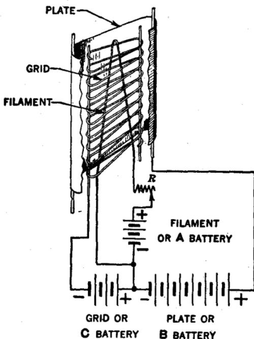
FIG. 14.—Schematic diagram showing triode connection to battery.
