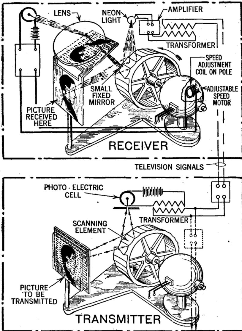
FIG. 6—Simplified view of a mechanical television system.
