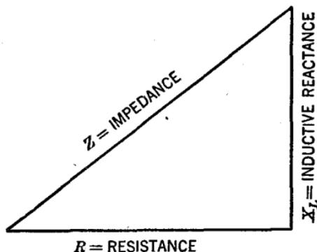
FIG. 11.—Illustrates vector relation between the inductive reactance and the resistance. To obtain the impedance: Resistance  $R$  (in ohms) is laid off horizontally; the inductive reactance  $X_L$  (also in ohms) is laid off to form the perpendicular. Measure the hypotenuse (in the same scale) which gives the impedance of the circuit in ohms. This triangle is variously referred to as the impedance triangle, vector diagram or impedance calculator.
