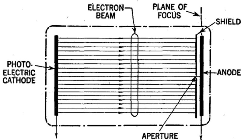
FIG. 23—Principle elements of Fansworth's "image-dissector" transmitting tube.
