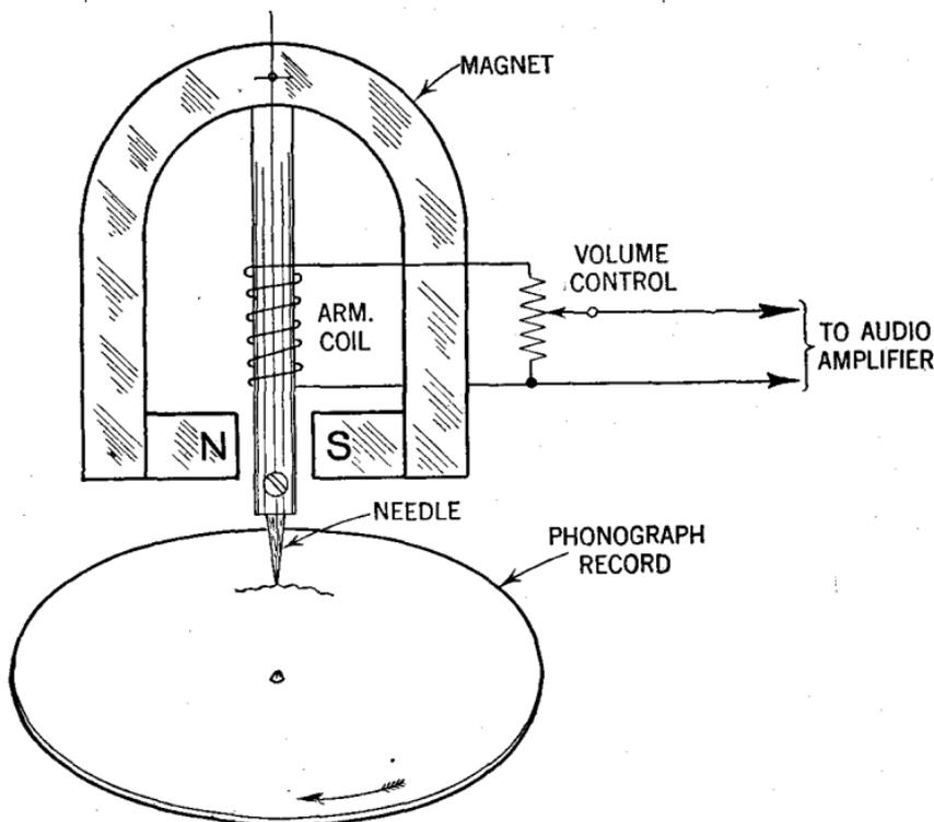
FIG. 3—Simplified layout of a phonograph pick-up.
