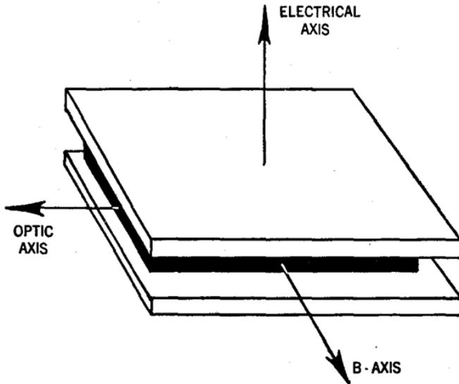
FIG. 13—Mounting of the crystal.
