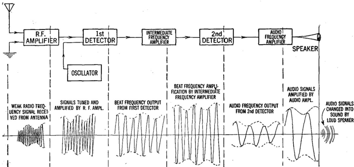
**FIG. 6—**Combination diagram showing arrangement of the different units of a typical super-heterodyne receiver with wave chart indicating how the radio signals are modified by each unit, that is, how the inaudible signals first picked up by the antenna undergo successive changes en route to the loud speaker.
