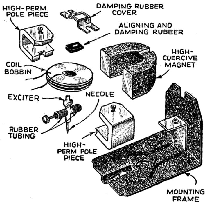
FIG. 4—Parts of modern rubber damped pick-up.
