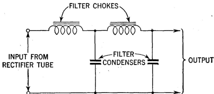
FIG. 6—Choke-input filter.
