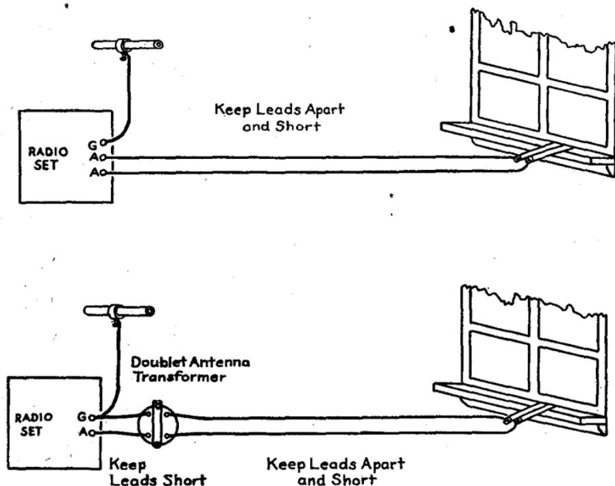
**FIG. 7**—Showing method of carrying antenna leads through the windows—using either porcelain tubes or flexible lead-in strips. Upper figure shows connections where antenna transformer is embodied in the radio receiver, and the lower, where it is connected outside. Transmission lines must be well insulated and stand off from the walls, as well as kept away from wires, drain pipes and other metallic surfaces and conductors.
