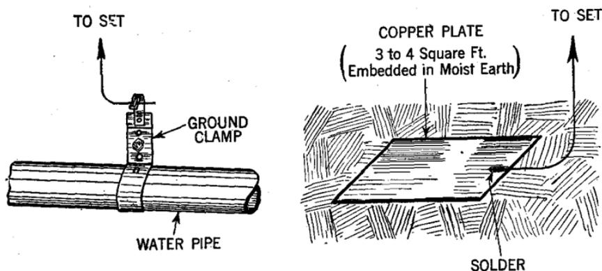
FIGS. 10 and 11—Two methods of ground connection.
