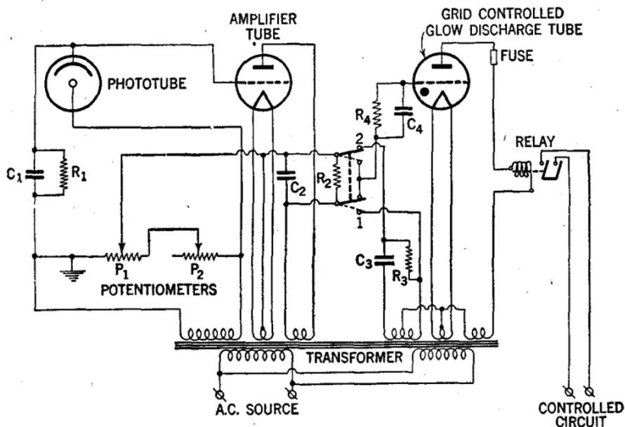
Fig. 10.—Wiring diagram of relay shown in fig. 9.
