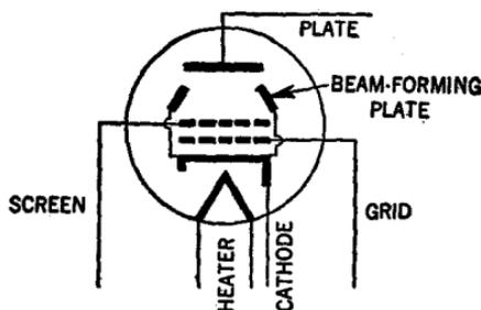
FIG. 19.—Conventional representation of beam power tube.
