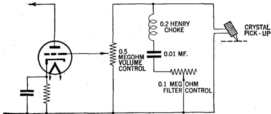
FIG. 13—Method of connection for phonograph pick-up.
