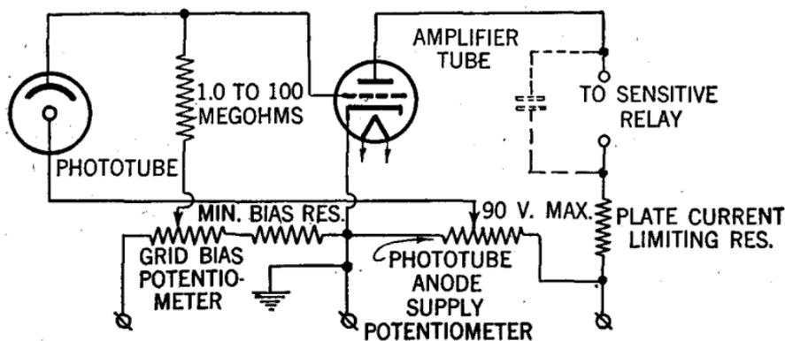
FIG. 27.—Typical relay circuit employing gaseous type phototube.
