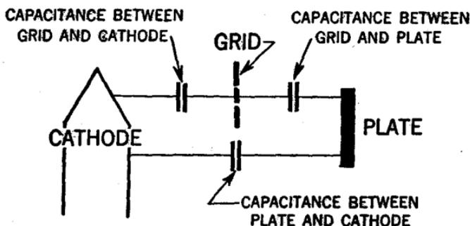
FIG. 16.—Diagram showing inter-electrode capacitances in a triode.
