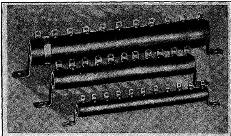
FIG. 14—Typical receiver power supply resistors.
