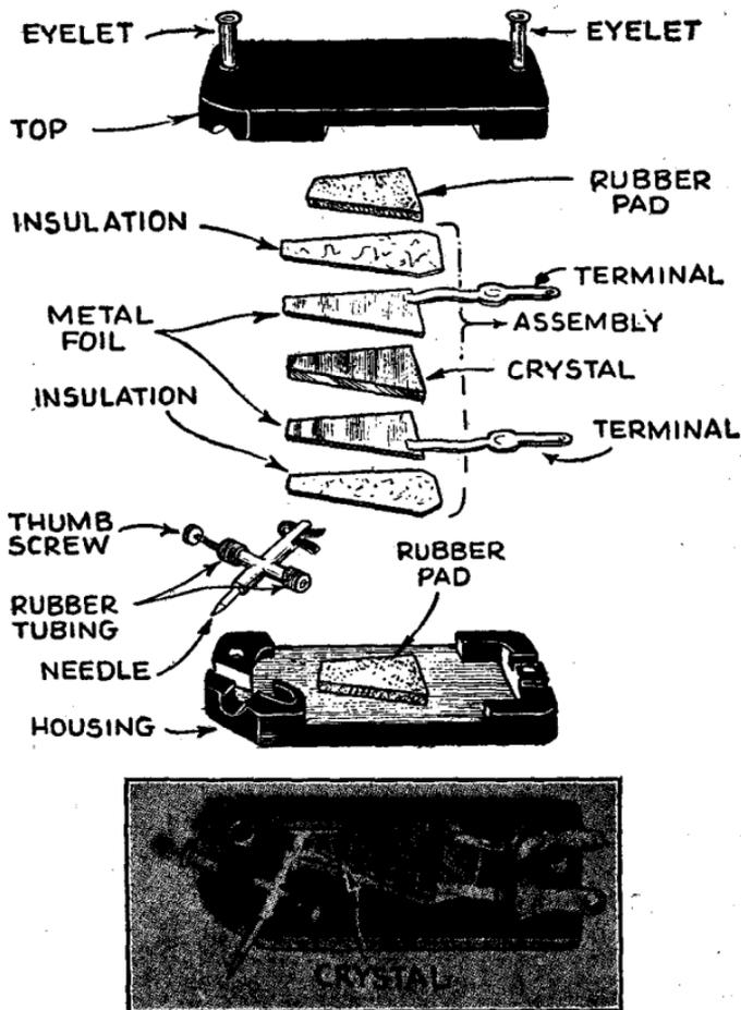
FIG. 6—Parts and assembly of crystal pick-up.
