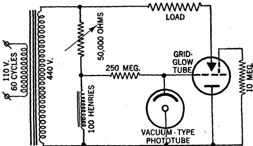
FIG. 47.—Grid-glow relay circuit A. C. operation.
