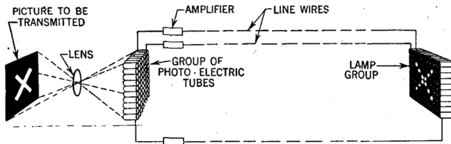
**FIG. 3—**Diagram of an early television system. At the transmitting end light is converted into electrical energy which when amplified will energize a magnetic shutter or similar device at the receiving end causing a reproduction of the picture. Each photo-electric cell must be individually converted to its correspondingly remotely located light element. In the case under consideration therefore, approximately 80 wires will be necessary.
