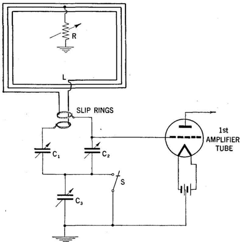
**FIG. 5—Circuit of Bellini Radio direction finder.**
