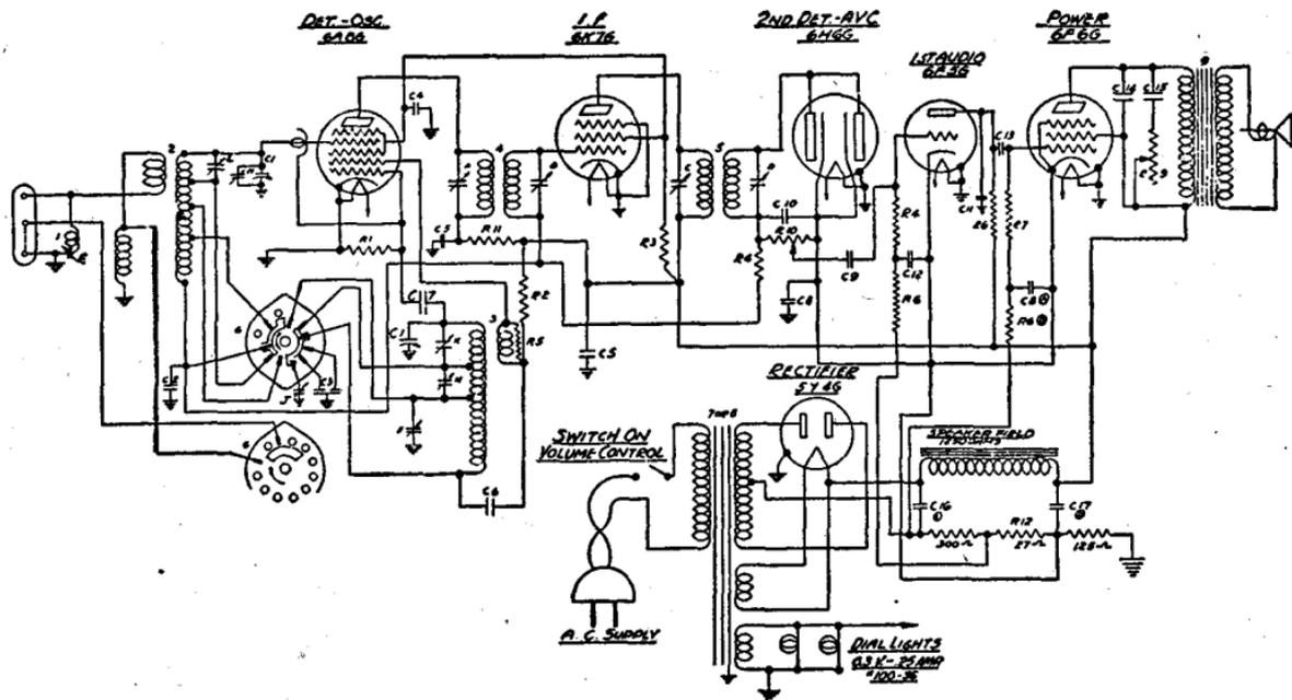
FIG. 5.—Schematic circuit diagram of a 6-tube superheterodyne, 3-band radio receiver. (Zenith Models, 6-S-203, 6-S-222, 6S-223, 6S-229, 6S-239, 6S-241.) *I.f.* frequency, 456 kilocycles. In locations subject to code interference adjust wave trap marked (E) for minimum interference with antenna connected and receiver operating in broadcast band. Line voltage 117 volts, a.c. 50 to 60 cycles. Power consumption 65 watts.
