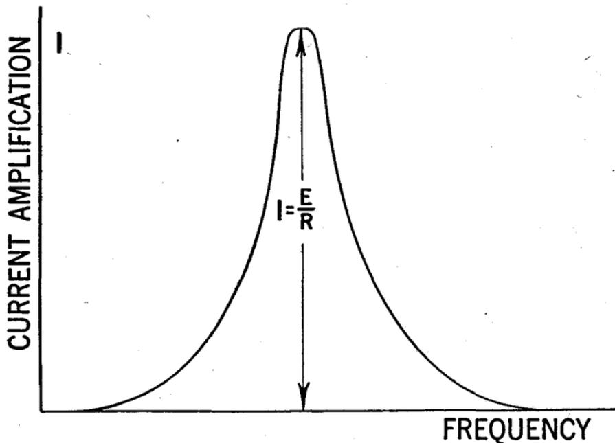
FIG. 5—Typical current resonance characteristic.
