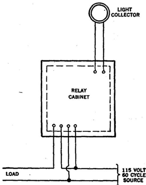
FIG. 6.—Wiring diagram of illumination control unit.
