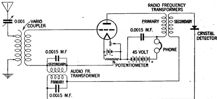
FIG. 28—Diagram showing typical reflex circuit.
