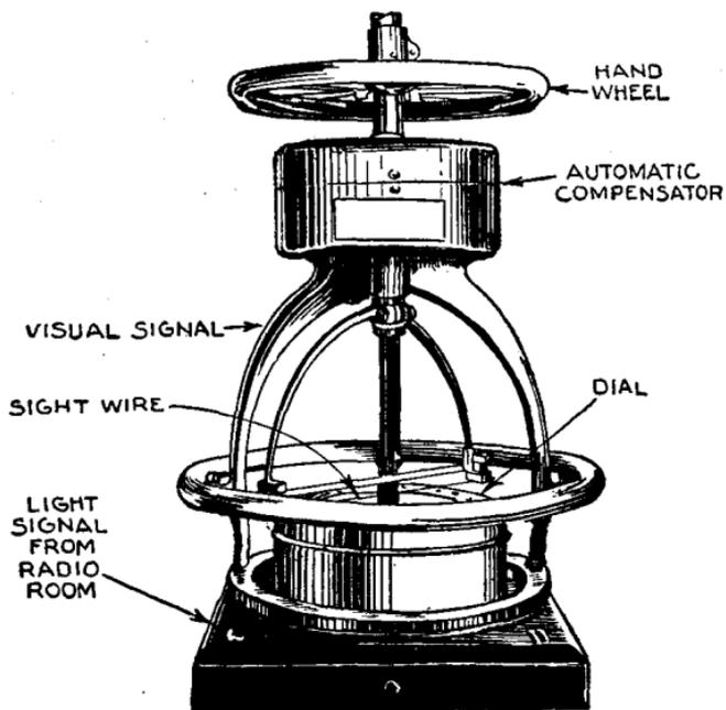
**FIG. 8—Kolster compass and compensator arrangement.**
