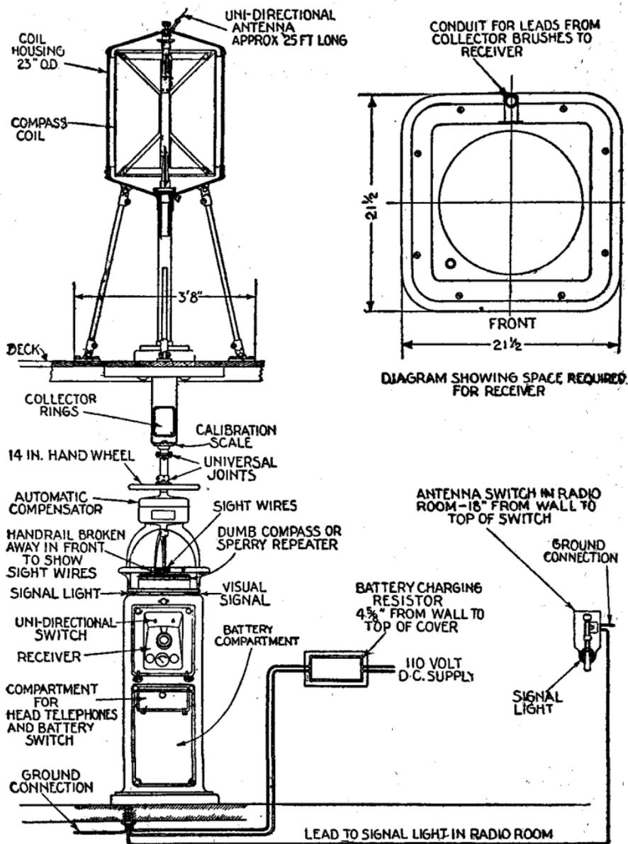
FIG. 3—Kolster radio compass installation.
