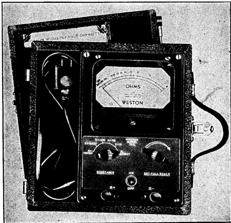
**FIG. 9**—Panel view of Weston Model 763 ohmmeter.
