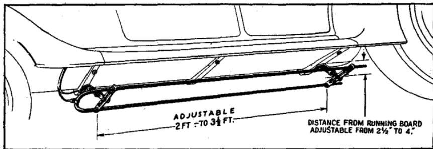
FIG. 5—Di-pole antenna and method of assembly.
