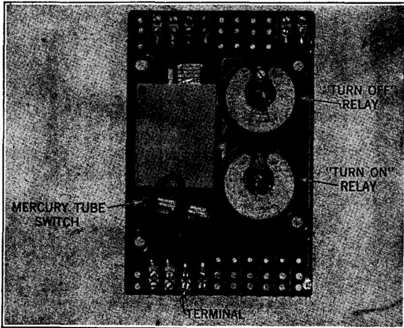
FIG. 5.—Illumination control unit, cover removed.
