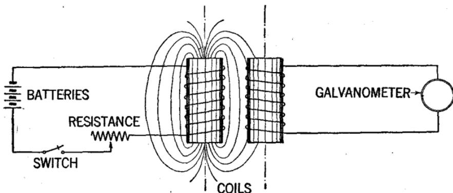
**FIG. 7**—Diagram showing the action of mutual induction between two coils; the one including a source of electrical energy and a switch, the other a current measuring instrument but having no source of electrical energy. During the increase or decrease in strength of current as on closing the switch the current is induced in the secondary circuit. This secondary current is flowing in a direction opposite to that of the primary current.
