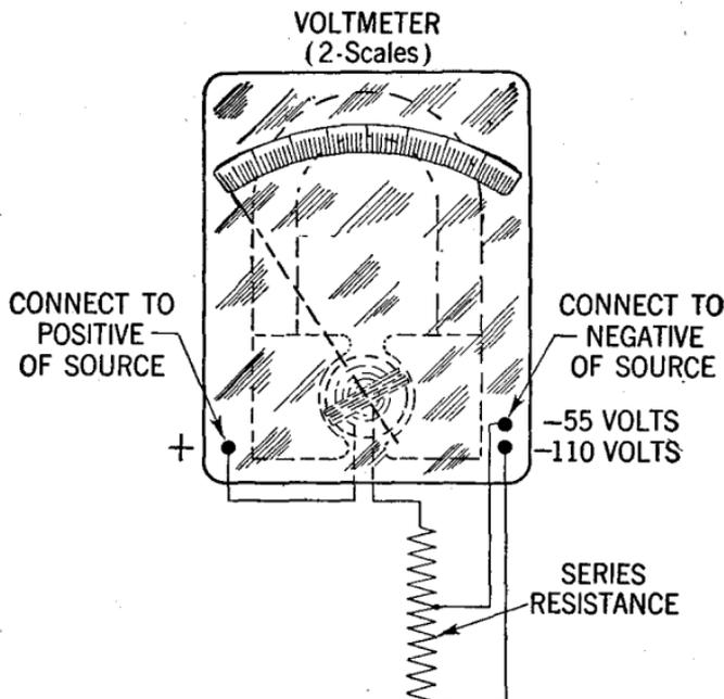
FIG. 8—Connection of multiplier resistance to 2-range voltmeter.
