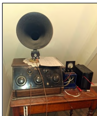
Above: Freed Eisemann 5-valve battery radio with Amplion horn, Philips B- battery eliminator and dual 6-Volt SLA A-battery. Offers?
