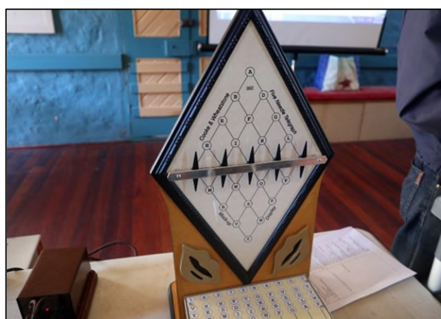
Above: Closer view of the dial of the 5-needle telegraph and keyboard.
