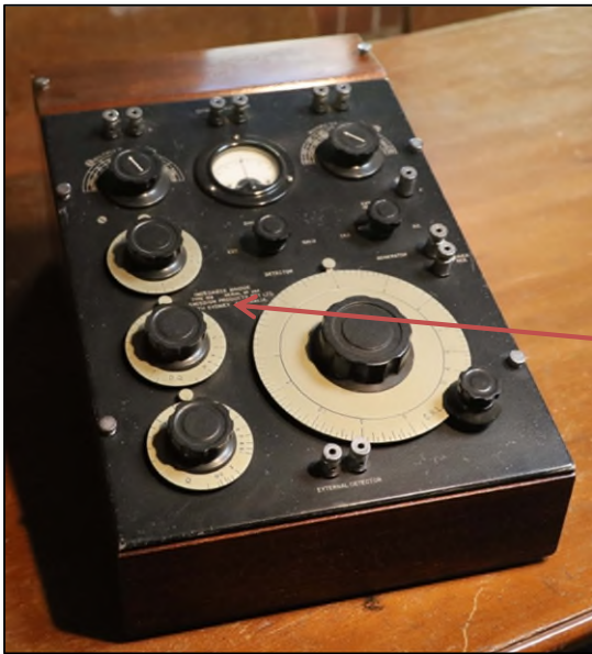
Above: Impedance Bridge by Transmission Products Ltd. -
