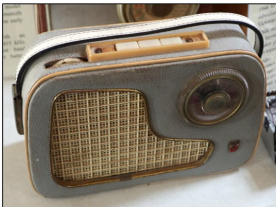
Above: The Philips “Skipper” Model 196 valve portable radio, made when transistor portables were coming onto the Australian market. Many manufacturers at this stage produced both valve and transistor models to try for full market coverage.
