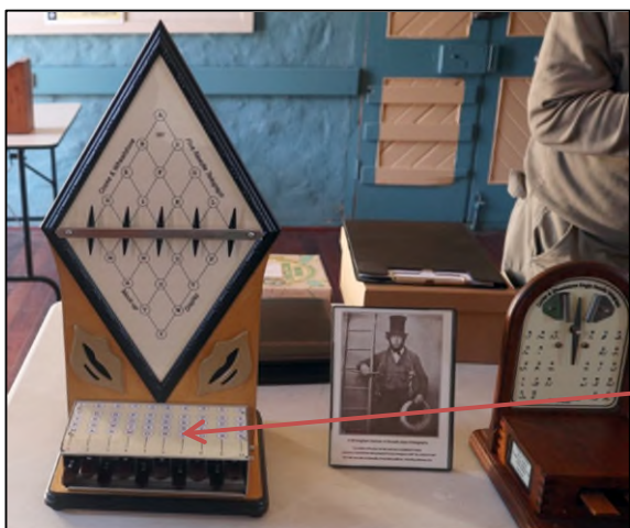
Above: Cooke and Wheatstone “5-Needle Telegraph”
