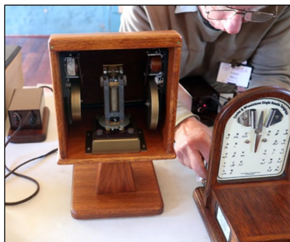
Above: Receiver box (wooden sound amplifier) for the single-needle telegraph.
