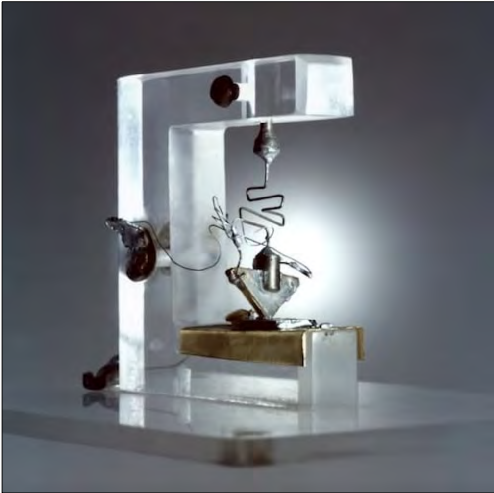
The point-contact transistor was developed by Brattain with Bardeen and Shockley. (Image used courtesy of Bell System Memorial)
