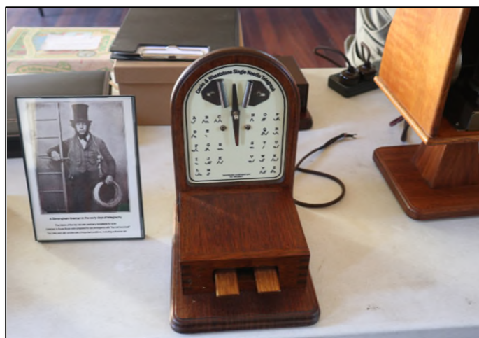
Above: Cooke and Wheatstone “single needle” telegraph (left and right needles make a slightly different note when hit.)
