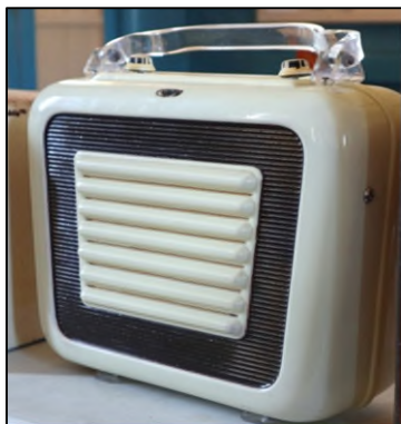
Above: "Operatic" Model 38P (1954) 5 valve portable radio with plastic case and clear handle.
