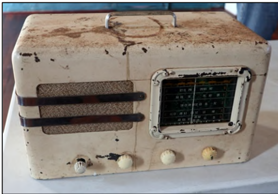
Above: Reg George started making 6-volt vibrator radios using two-volt heater valves with a tuned RF stage, in metal cabinets with the "Standard" name plate fixed on the back,
