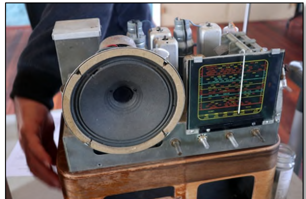
Above: Chassis of the T29 is in excellent condition EXCEPT for the 9v Vibrator AND an apparent 240v AC mains cable in there together!
