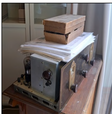
Above: Pilot Super-wasp battery short-wave receiver with plug-in coils and documentation. Make an offer
