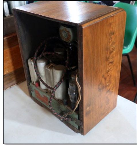
Above: Rear view of the radio on left, showing 6A7, 6D6, 6B7, 42 & 80 valves.
