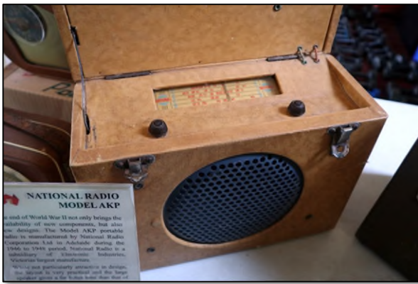
Above: The model AKP Portable valve radio was manufactured by National Radio Corp. in Adelaide (1946-48.) Whilst not very attractive, it was a good performer with a larger speaker with better tone than later transistor radios of a similar size.
