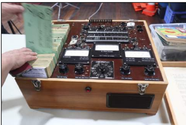
Above: The FUNKE model W20 (Germany, 1955) Valve tester from the HRSASA Valve Bank. This was the late Duncan McDonald's favourite machine! Note on the left, the blue cardboard "punch cards" that are used to calibrate the machine to test each individual valve type.
