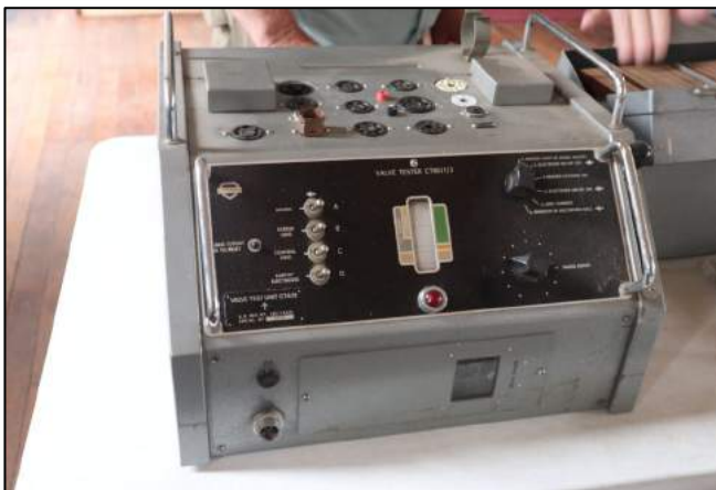
Above: The 1954 Australian-made MULLARD model CT80/1/3 (or CTA 20) was a top-of-the range valve tester by the people who make the valves! Almost all valve testers usually require the manual setting of a number of switches and dials appropriately for each valve. However this tester uses a large set of punched cards which automatically program the tester for a particular valve.
