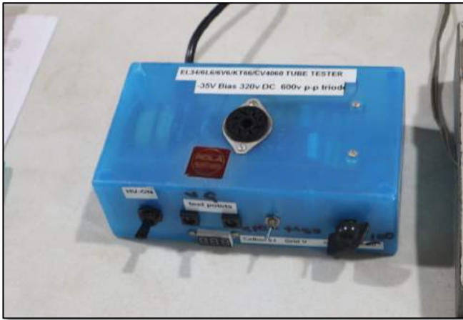
Above: A ROLA branded single-base, very specific tester for audio valves, EL34, 6L6, 6V6, KT66, and CV4060.
