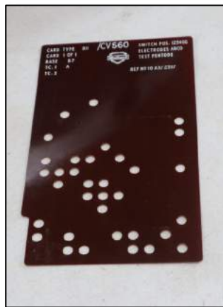
Above: The 1954 Australian-made MULLARD model CT80/1/3 (or CTA 20) was a top-of-the range valve tester by the people who make the valves! Almost all valve testers usually require the manual setting of a number of switches and dials appropriately for each valve. However this tester uses a large set of punched cards which automatically program the tester for a particular valve.
