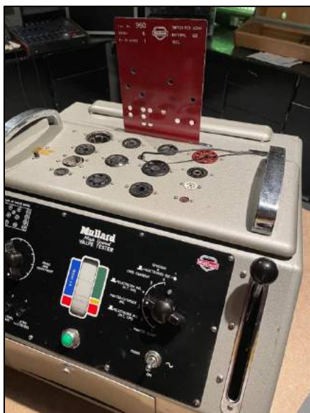
Above: The Mullard with the punch card in place above the test sockets,
