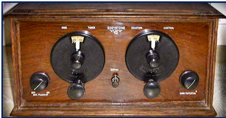
Above: The Eddystone “Atlantic Two” (2 valve) Model short-wave receiver from 1927
