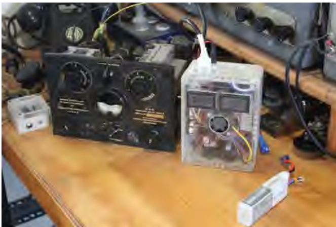
Australian-made Transceiver Model 108 Mark II being bench tested – Photo: Stephen Parker
