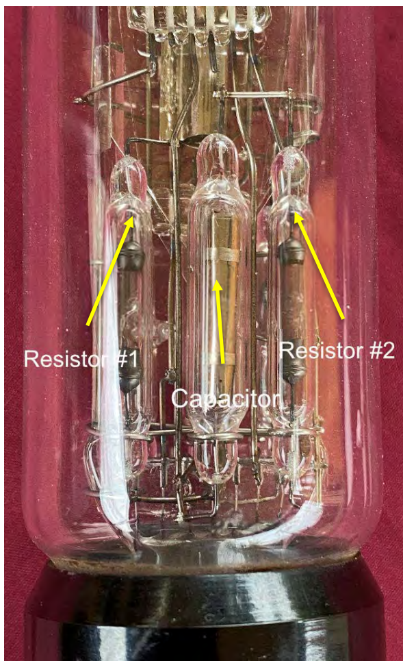
Above: Two Resistors and one Capacitor inside each tube – Repeated on the reverse side.
