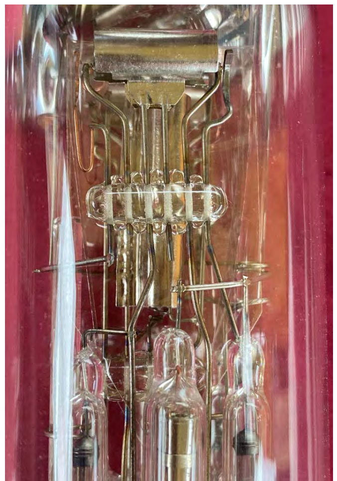
Above: 3 Triodes are located above the passive components. Two triodes mounted horizontally and one vertically between them.
