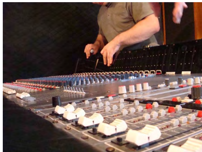
The fully restored, 40 track Harrison MR4 mixing console
