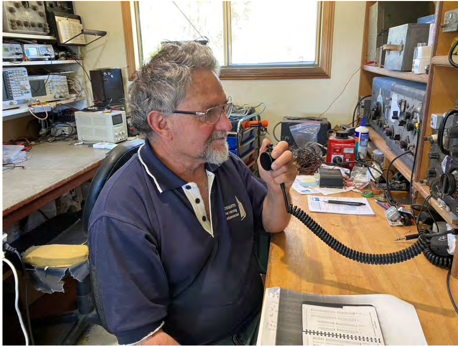
Phil at the controls of a BC348 receiver (made by Stromberg Carlson.) The transmitter is a ART13 (made by Collins) usually used in B17s, and the USAF “Liberator” and the larger “Flying Fortress”.
