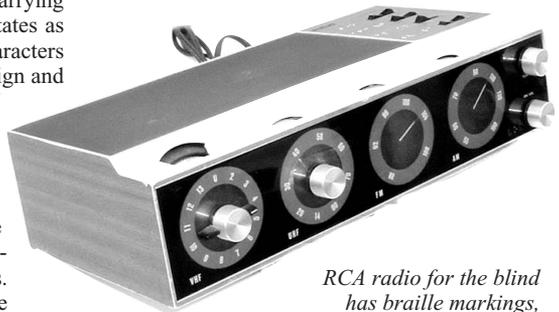
*RCA radio for the blind has braille markings, tunes AM and FM as well as VHF and UHF TV audio.*
